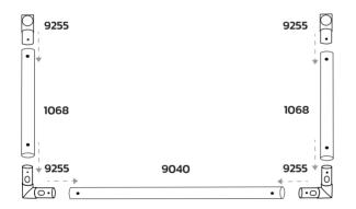
Assemble the crossbar and the upright section, attaching 9040 & 1051 to connectors.
