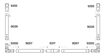
Assemble the crossbar and the upright section, attaching 8975 & 9057 to connectors.
