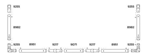
Assemble the crossbar and the upright section, attaching 9064, 9071, 8968 & 8951 to connectors.
