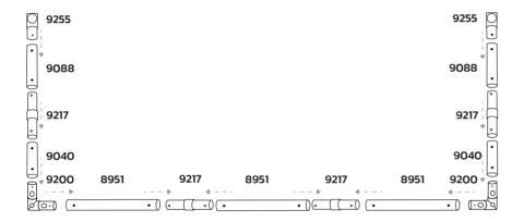
Assemble the crossbar and the upright section, attaching 9088 & 8951 to the connectors.
