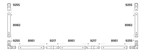
Assemble the crossbar and the upright section, attaching 9088, 8968 & 8951 to connectors.
